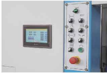
* Touch Screen which can set board size and finish orientation automatically.
