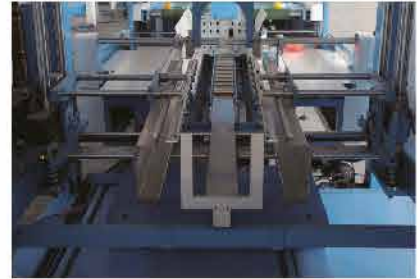
* Turning Device driven by servo motor
